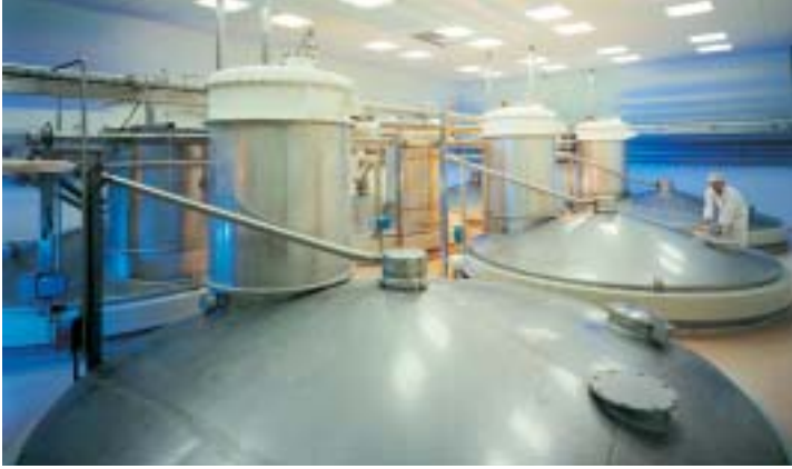
Top of 100 m 3 milk powder silos. Silos are equipped with automatic self-cleaning filters
