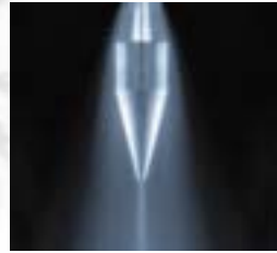
Reverse jet nozzle for SANICIP™ CIP-able bag filter and IFD™ dryer
