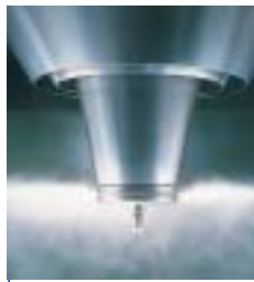
Rotating atomizer wheel in operation
