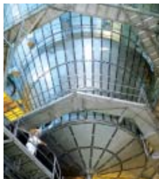
MSD™ Dryer with removable insulating panels
